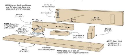
**Simple Machine.** My solution involves taking advantage of a lever to apply pressure to my workpiece as I make a cut. The lever is made from plywood and pivots on a screw that attaches it to my sled back.
