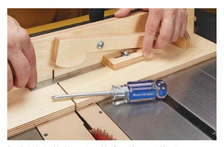
An adjustable stop block is easy to position for making repeatable cuts.
